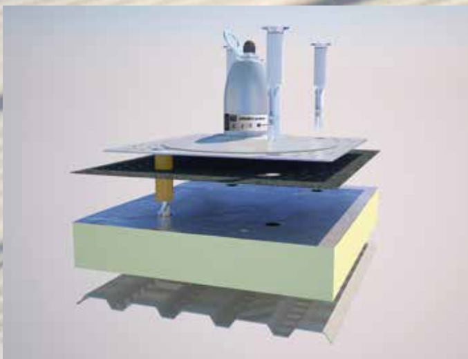
Toggle Fixing Method
