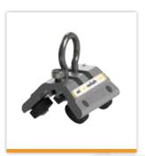
Attachment carriage (Part code: 7241006) – enables the user to connect to the system and enjoy complete hands-free movement along the rail. It features a stainless steel parking lock for work positioning tasks and aluminium, nylon coated wheels. A stainless steel shackle enables connection of a karabiner hook and pivots to enable best functionality at any angle of take off. Min strength 15kN (3300lbs)
